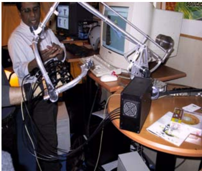
Fig. 3 The upper photograph shows one of the various types of Head Mounted Display (HMD) available today. The lower photograph shows a haptic force-feedback device. Just as HMDS, haptic systems come in a large variety of configurations. Their application in conjunction with HMDs or other forms of VR allows interaction with virtual reality rendered objects
