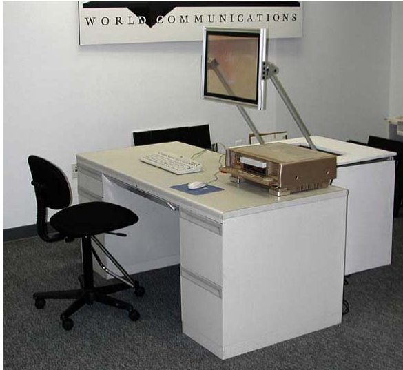
Fig. 5 LifeVision desk-top system by Intrepid World Communications. Note the compactness of the device (the cuboid box behind the operator's desk) making it immensely applicable in a variety of limited space settings. The flat screen folds down for transport. However, compared to the MIRROR device by Ethereal Technologies, the LifeVision system is more complex and less suitable for field deployments or deployments to the regions where technical assistance may not be readily available. The box on the right side of the desk is a 3-D videorecorder.
