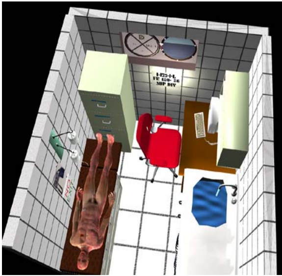
Fig. 11 VR-based medical telepresence system. The immersive VR (CAVE) environment represents the exact environment of the sick bay aboard US Coast 270ft cutter. The bay is capable of virtual movement (pitch and roll) controlled by the CAVE operator. Like in a real ship, sea sickness can be induced by varying the intensity of the “virtual storm.” While the virtual sea state creates 5m (rough ship waves), the training personnel begins to roll their bodies and compensate for the “movement of the ship” the despite completely stationary floor. The patient is the “first-eyer” texture map (VR) of a badly burned survivor.
