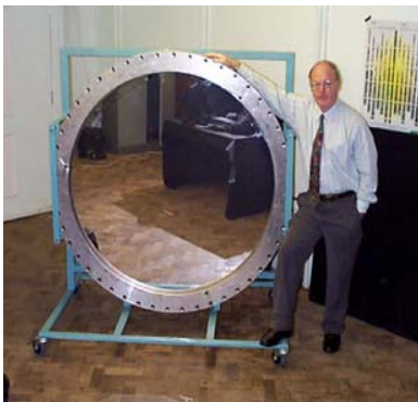
Fig. 4 The stretchable membrane mirror system - a relatively simple but very effective autostereoscopic device.
