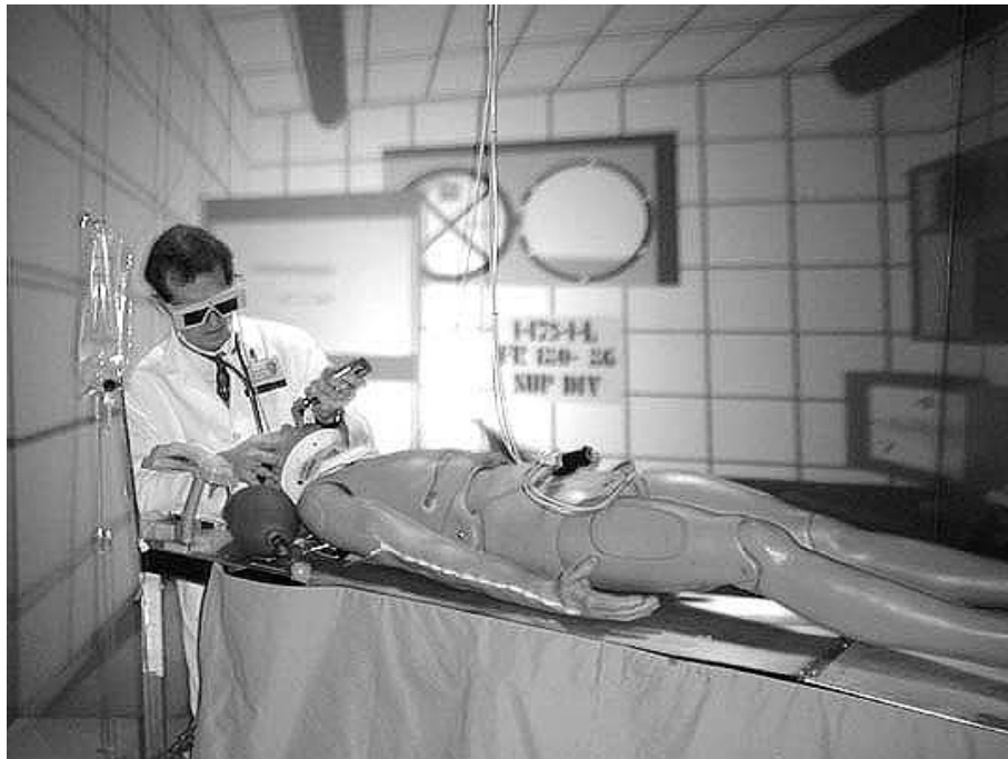
Fig. 1 Human Patient Simulator (METI Version “B”) in action. The computerized mannequin is capable of faithful reproduction of several diseases. It also responds to administration of drugs and I.V. fluids (note the saline solution in the bag attached to the pole to the left), and several procedures such as defibrillation, insertion of laryngoscope (procedure shown in the picture), catheters, etc. Here, the physician-instructor demonstrates airway management in a victim of a major accident aboard a ship. As in human patients, the vital signs correctly generated by the HPS are displayed on a monitor whose screen is seen on the right side. HPS systems are ideal for training under near “real life” conditions and, as human patients when the treatment is incorrect, can “suffer” of adverse effects or even “die”. The mannequin is surrounded by the virtual reality environment (CAVE TM ) hence the goggles worn by the physician. The goggles allow perception of three dimensions and proper perspective.
