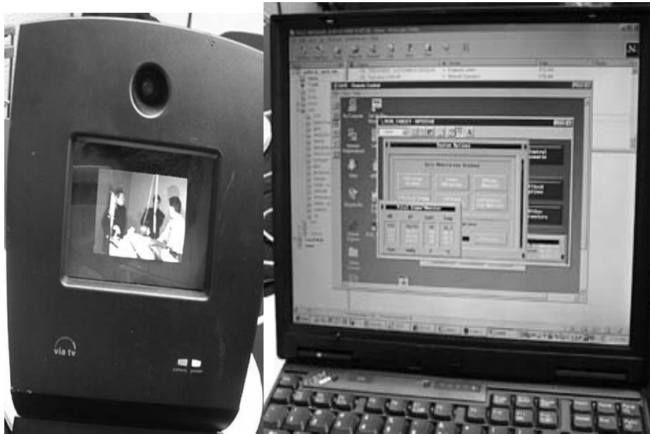
Fig. 3 On the left, Via TV Phone (8x8, Inc.) unit showing the instructor (right side of the unit's screen) and two trainees at the simulator site. The remote trainees (see Fig. 2) observe both the simulator and the instructor on the screen. On the right, a laptop computer with HPS remote control interface and vital sign display. Vital signs can be presented either as numbers or, as on a standard hospital monitor, in form of continuous lines with numerical values in a side bar. Monitor sounds (beeps, alarms) can be also generated. Both the remote trainees and the instructor can control the HPS. In a typical training session, the instructor sets the scenario (shock, cardiac arrhythmia, severe burn, asthmatic attack, etc.), then cedes control of the HPS unit to the remote trainee(s) whose task is to manage the case using remote control of the machine. Remote commands instruct the HPS to perform electronically the required procedures (such as defibrillation, intubation, placing of catheters) electronically. Once appropriate drugs are selected and their dose determined by the trainees, these can be also "administered" via remote control. Although remote access to the simulator eliminates haptic (force) feedback and the ability to train manual procedures, even this form of training is intellectually challenging and its pace, just like in the real life, can be very brisk. The real time presence of an expert instructor (either at the simulator site or, just as that of the trainees, at a remote but different location) allows immediate correction, advice, and debriefing. Scenarios can be re-run as many times as required assuring proper mastery of the involved treatment algorithms.
