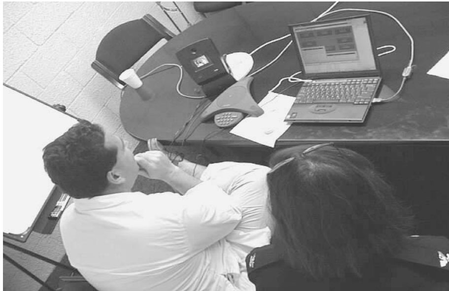
Fig. 2 Two physicians at a remote location (Puerto Rico) during a training session on a Human Patient Simulator located in Ann Arbor, MI, nearly 3000 miles away. The laptop computer screen contains two windows: one permitting remote control of all simulator functions, and the other displaying all pertinent physiological data of the “patient”. The star-shaped device on the table is a standard conference telephone for hands-free voice communication. Left of the telephone stands a mini video screen (Via TV Phone, 8x8, Inc.) permitting direct observation of the HPS and its physical behavior (such as movement of the chest). Apart from the laptop computer (IBM Thinkpad), all other elements of this set-up can be bought at a very moderate price at almost any electronic supplies store. Plain Old Telephone (POTS) – based connection (two lines) and a 56 Kb modem are used to access the Internet. It is most likely the simplest and cheapest solutions to advanced distributed medical training based on HPS technology that is accessible to virtually anyone.
