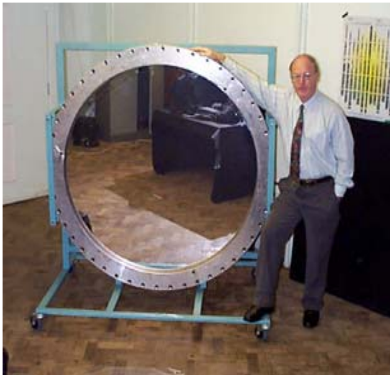
FIG. 1 Stretchable mirror (early version) used in the pilot technology demonstrations described in the text. Courtesy EtherealTechnologies, Inc., Ann Arbor, MI
