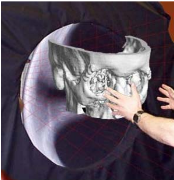
FIG. 3 MIRROR 3-D visualization of a human cranium as an example of facilitation in planning reconstructive surgery following major trauma. Courtesy Ethereal Technologies, Inc., Ann Arbor, MI
