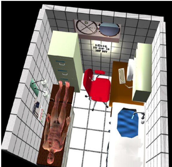
FIG. 5 VR-based medical telepresence system. The immersive VR (CAVE) environment represents the exact environment of the sick bay aboard US Coast 270ft cutter. The bay is capable of virtual movement (pitch and roll) controlled by the CAVE operator. Like in a real ship, sea sickness can be induced by varying the intensity of the “virtual storm.” When the virtual sea state reaches 5 (moderate waves), the training personnel begins to roll their bodies to compensate for the “movement of the ship”, despite completely stationary floor. The patient is the “first-ever” texture map (VR) of a badly burned survivor.
